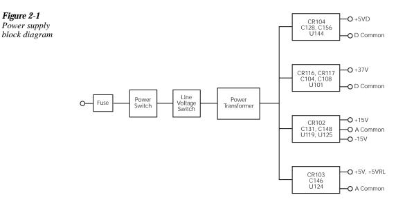
AC power is applied to the AC power module receptacle (J1009). Power is routed through the line fuse and line voltage selection switch of the power module to the power transformer. The power transformer has a total of four secondary windings for the various supplies.
